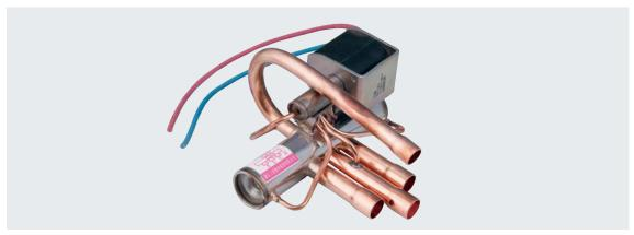
SHF (G) series four-way valves are especially applicable for heat pump systems including high-end and high-efficient unitary and room air conditioners to realize switching between cooling mode and heating mode by changing the flow path of refrigerant.
