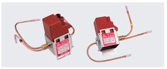
FDF series 2-position 3-way solenoid valve is used in dual temperature/double control household refrigerators and similar small scale refrigeration systems for switch of refrigerant flow path.
