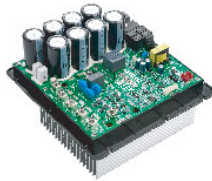
Sanhua Inverter Controller
